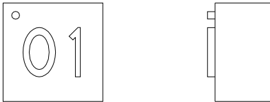
Figure 437 Node address jumper - front and side view
