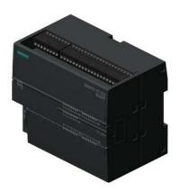
SIMATIC S7-200 SMART, CPU SR40, CPU, AC/DC/relay, onboard I/O: 24 DI 24 V DC; 16 DO relay 2A; Power supply: AC 85-264 V AC at 47-63 Hz, Program/data memory 40 KB
