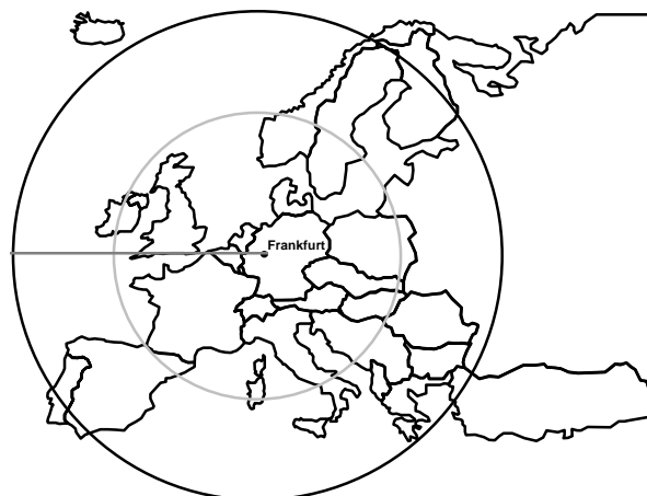
Figure 3 Receive radius of DCF atomic clock radio near Frankfurt
