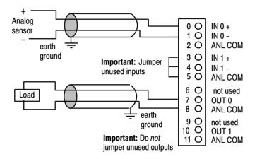
As an alternative, you may wire input transmitters having 2-wire, 3-wire, or 4-wire inputs in a single-ended current-loop configuration.
