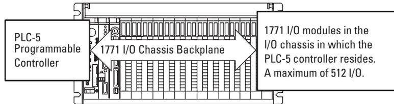
On-board remote I/O scanner ports are available on all PLC-5 controllers. On-board extended-local I/O scanner ports are available on some PLC-5 controllers. On-board ControlNet ports are available on some PLC-5 controllers. To provide a DeviceNet I/O scanner port to the system, you must add a 1771-SDN DeviceNet Scanner Module.
