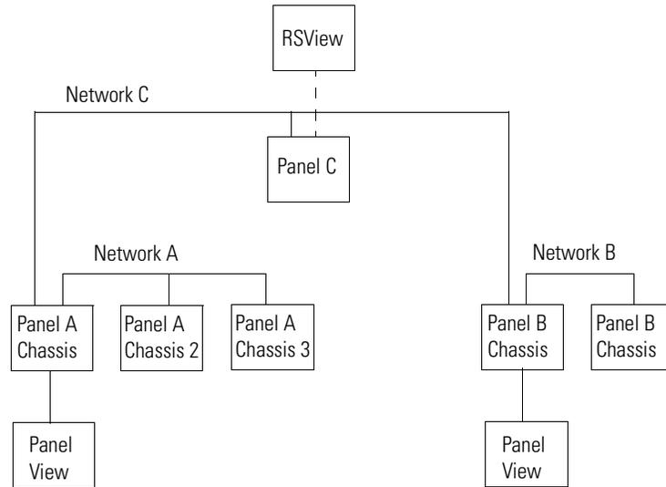
For a PLC-5 controller to control I/O modules, both the controller and the I/O modules must be directly attached to the same network.
