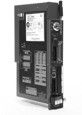
Every PLC-5 controller offers built-in, configurable ports for Data Highway Plus (DH+) or Remote I/O. A DH+ connection supports remote programming and information access, in addition to peer-to-peer communication between the PLC-5, other controllers, and devices. A Remote I/O connection supports real-time data exchange for I/O, operator interface, and other third-party devices.
