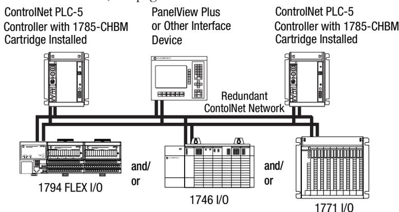
The PLC-5 Backup Communication Module, 1785-BCM, helps increase the fault tolerance of PLC-5 programmable controller systems controlling I/O on a remote I/O link by providing backup of the PLC-5 programmable controller.
