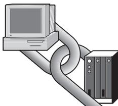
RSLinx software, 9355 series, is a communication server package that provides plant-floor device connectivity for a wide variety of applications. RSLinx software can support multiple software applications simultaneously communicating to a variety of devices on many different networks.
