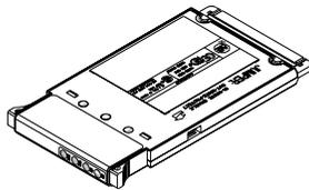
The ControlNet Hot Backup Module provides backup of ControlNet I/O. A secondary controller qualifies critical control information with the primary controller. Both controllers consume information from inputs and connect to outputs, but only the primary controller controls the outputs. The secondary controller establishes control of outputs if the primary controller shuts down.
