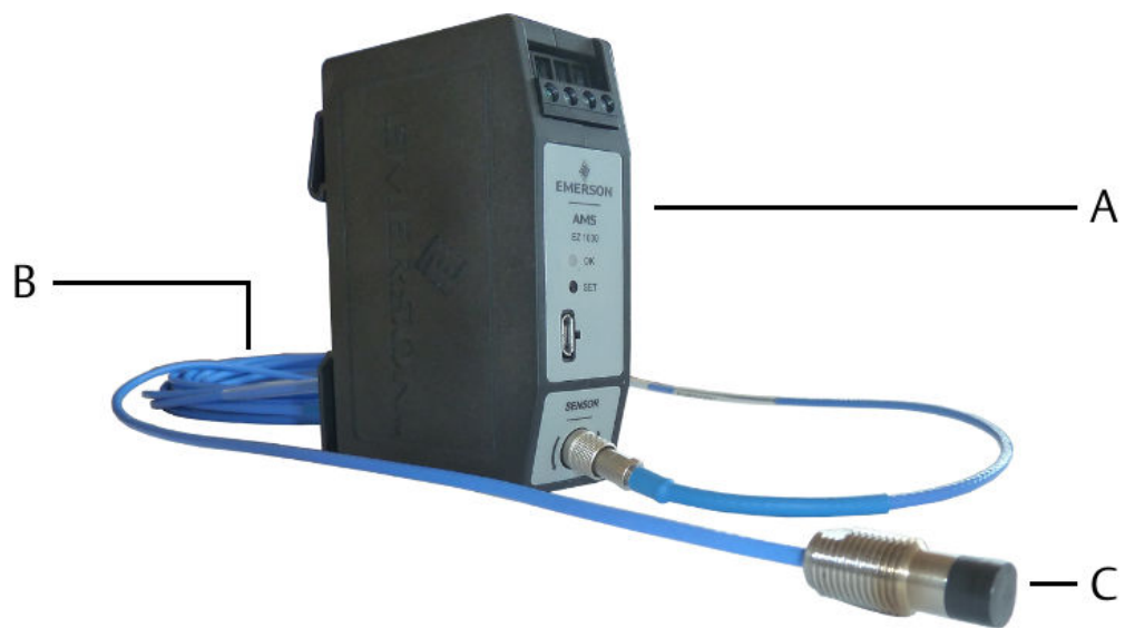
Figure 3-2: Eddy current measuring chain
