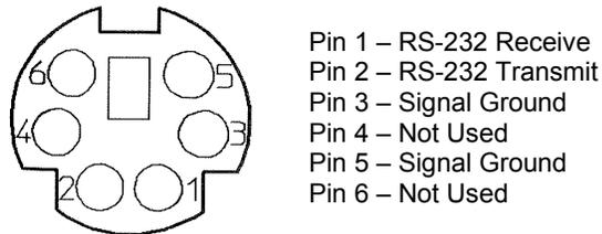
Figure 5-9—CPU Service Port (mini-DIN6F)
