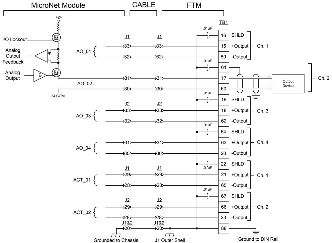
Figure 7-10—Analog Output and Actuator Wiring for an Analog Combo FTM
