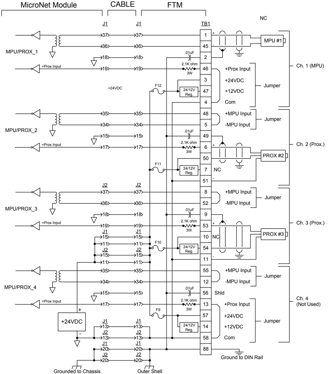
Figure 7-7—MPU/Proximity Interface Wiring to the Analog Combo FTM
