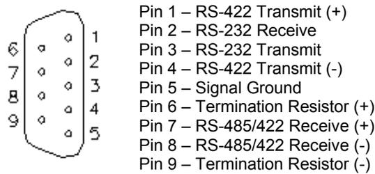
Figure 5-3—CPU Communications Port (DB9F)
