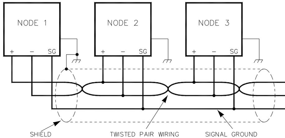
Figure 5-7—Preferred Multipoint Wiring Using Shielded Twisted-Pair Cable with a Separate Signal Ground Wire
