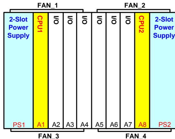
Figure 3-2—MicroNet Plus 8-Slot Chassis
