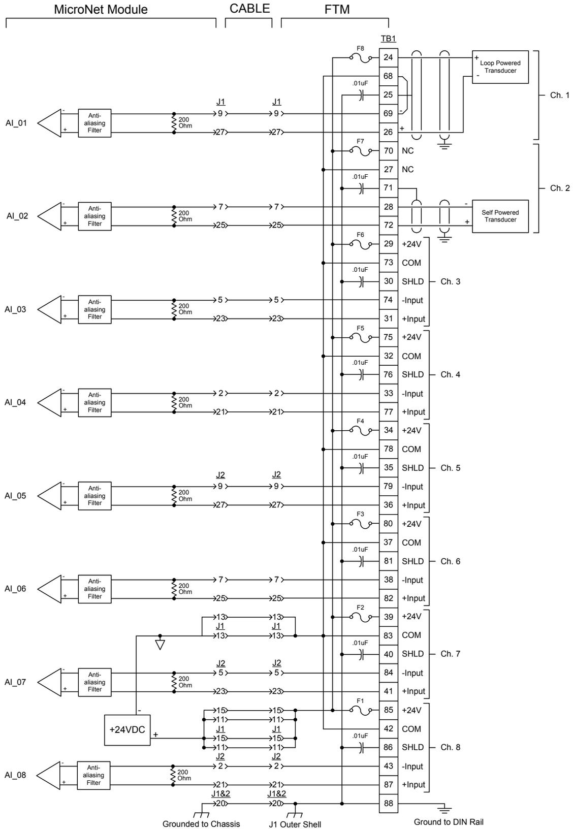
Figure 7-8—Current Input Wiring for an Analog Combo Module FTM
