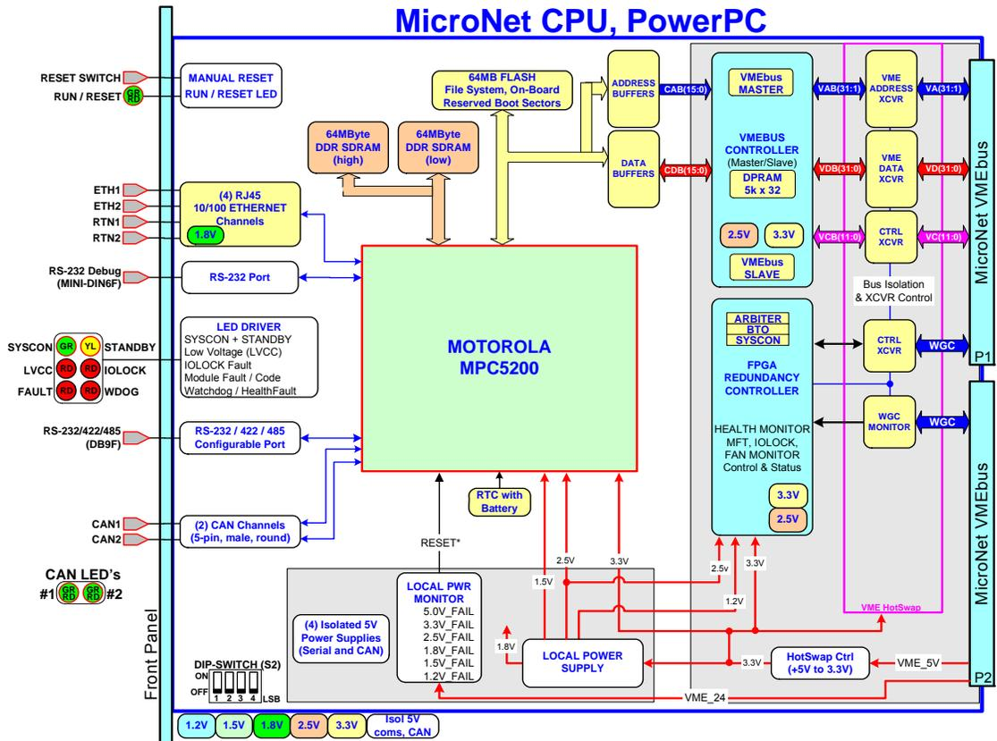
Figure 5-2—CPU Module Block Diagram
