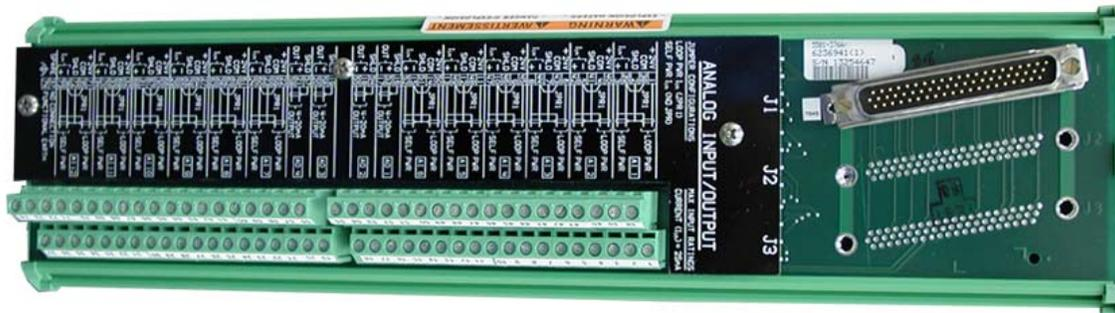
The 24/8 Analog FTM is used with the 24/8 Analog Modules (see Chapter 7 MicroNet module information and Appendix A for FTM part number). One MicroNet High Density Analog/Discrete cable is use to connect the FTM with the 24/8 Analog Module (see Appendix A for part numbers). There are twelve +24 Vdc connections available for sourcing 4-20 mA inputs. Each connection is protected with a 0.1 A fuse.
