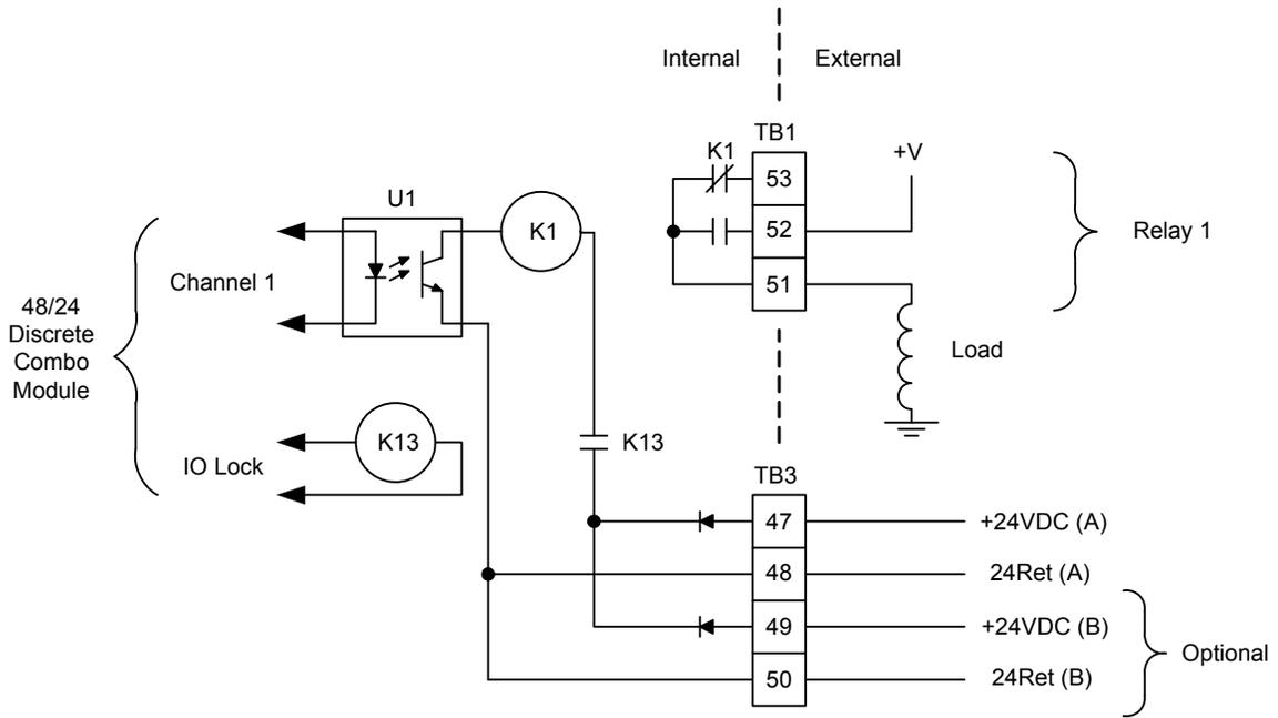
Figure 6-4—Relay Output Interface Wiring to a 24/12 Discrete FTM
