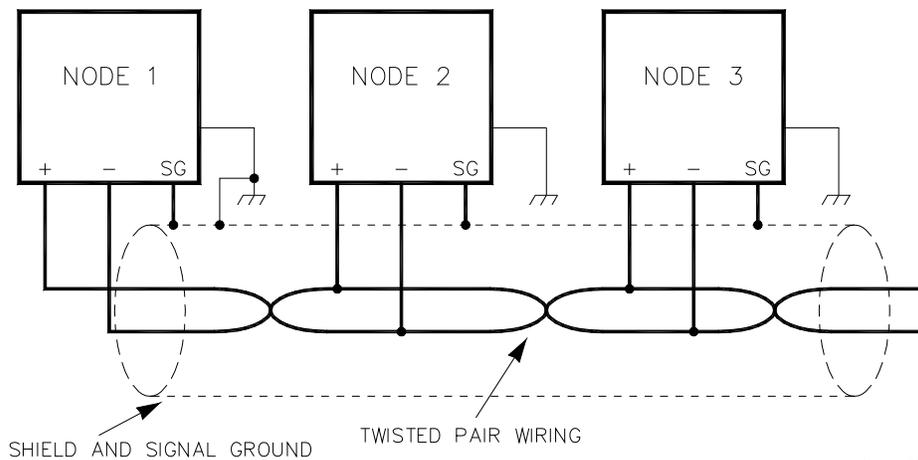
Figure 5-8—Alternate Multipoint Wiring Using Shielded Twisted-Pair Cable without a Separate Signal Ground Wire
