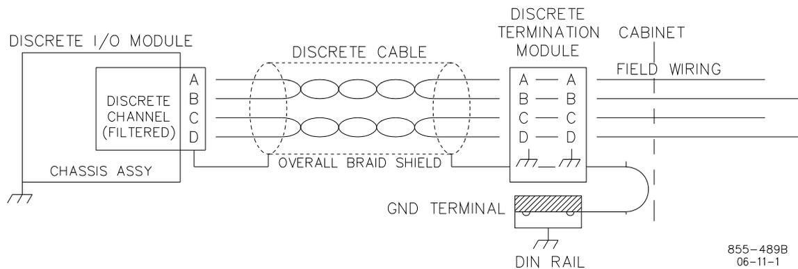
Figure 9-4—Discrete FTM Grounding Diagram Example
