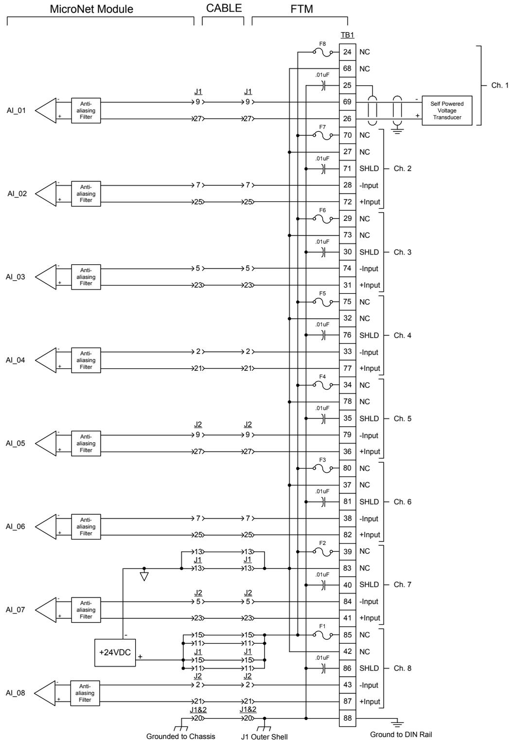
Figure 7-9—Voltage Input Wiring for an Analog Combo Module FTM
