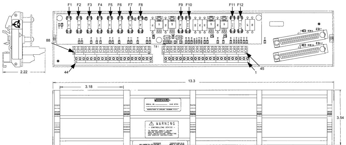
Figure 8-3—Analog Combo FTM Outline Dimensions
