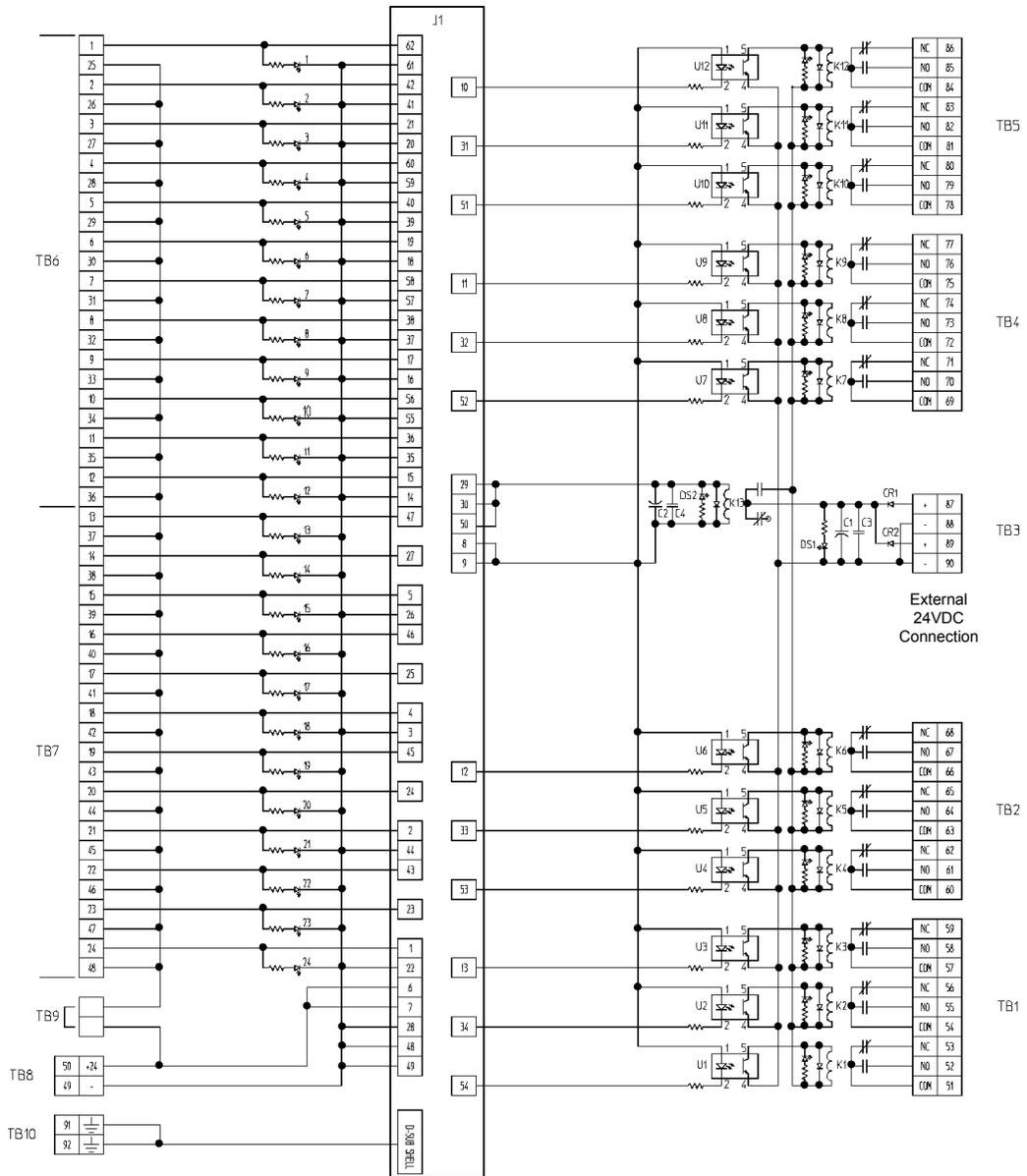
Figure 8-6—24/12 Discrete Module Schematic
