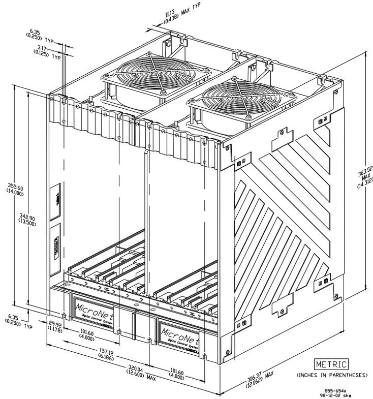
Figure 3-3—Outline Drawing of MicroNet Plus 8-Slot Chassis
