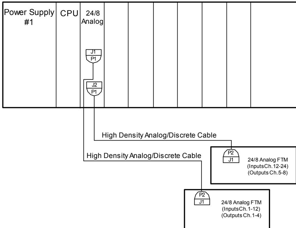
Figure 7-2—Simplex System Configuration Example
