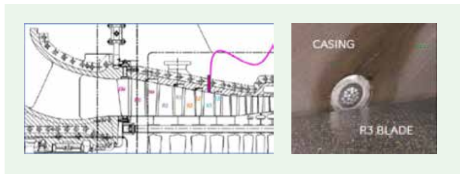
Figure 17: Sensor installation location on the GT compressor section
