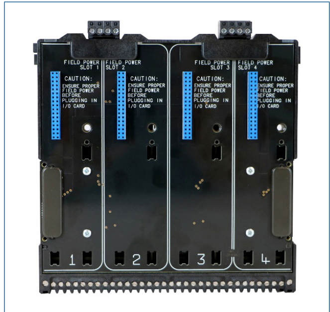
4-wide I/O card carrier with individual field power connections.
