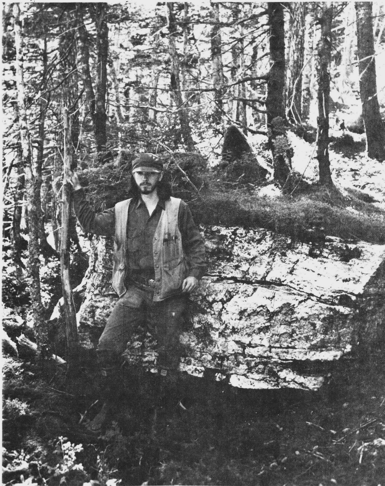
Figure 3. - Quartz float from the Big Croppings veins. A 5-foot sample across this vein (9S055) assayed 0.19 oz. gold per ton and 0.3 oz. silver per ton and contained no other significant metal values.
