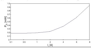
P[mW] Power dissipation in mW I<sub>L</sub>[A] Load current in the segment circuit in Amps
